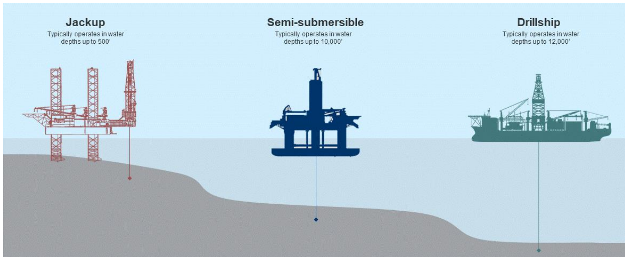
Figure 3: Main rig categories by water depth
